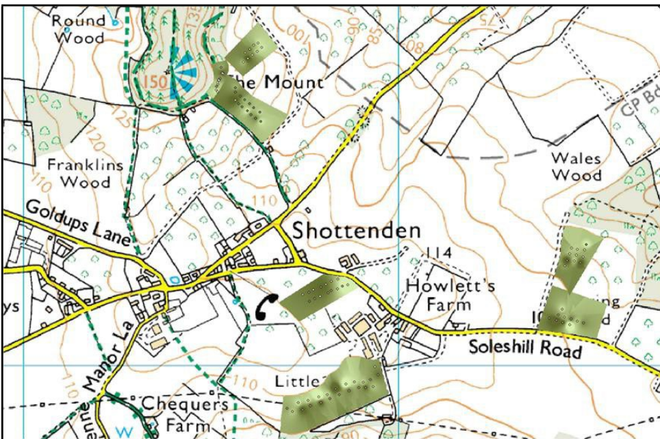
Figure 56. Site 6 map indicating soil C using data collected (the dots on the map) and interpolated to create a continuous surface using the inverse distance weighted (IDW) method on ArcMap (ArcGIS version 9.3.1 ESRI, 2009). Areas in a darker shade indicate higher levels of carbon. © Crown copyright / database right 2010. An Ordnance Survey / EDINA supplied service.
