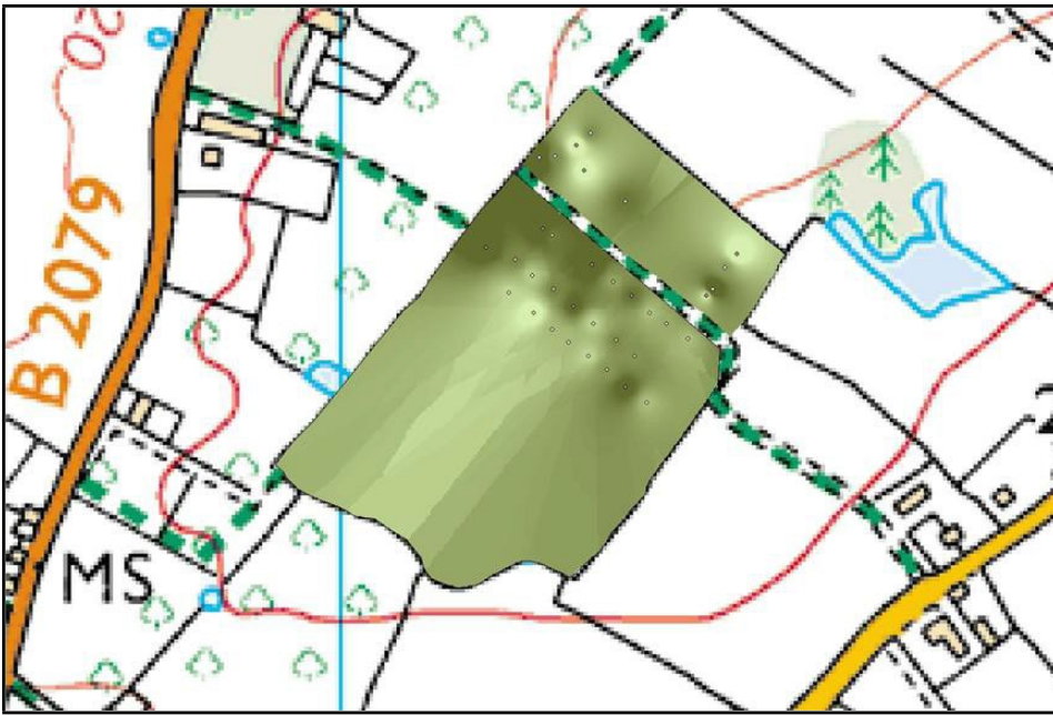
Figure 55. Site 5 map indicating soil C using data collected (the dots on the map) and interpolated to create a continuous surface using the inverse distance weighted (IDW) method on ArcMap (ArcGIS version 9.3.1 ESRI, 2009). Areas in a darker shade indicate higher levels of carbon. © Crown copyright / database right 2010. An Ordnance Survey / EDINA supplied service.
