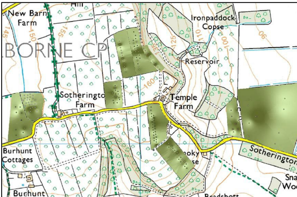
Figure 54. Site 4 map indicating soil C using data collected (the dots on the map) and interpolated to create a continuous surface using the inverse distance weighted (IDW) method on ArcMap (ArcGIS version 9.3.1 ESRI, 2009). Areas in a darker shade indicate higher levels of carbon. © Crown copyright / database right 2010. An Ordnance Survey / EDINA supplied service.
