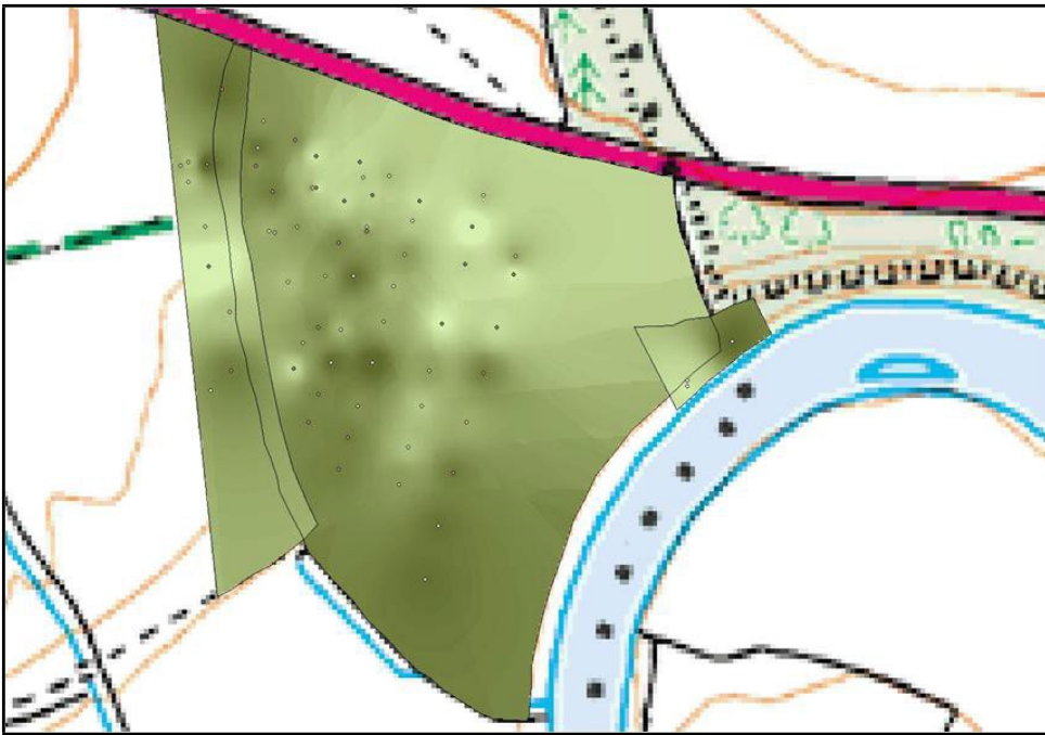
Figure 53. Site 3 map indicating soil C using data collected (the dots on the map) and interpolated to create a continuous surface using the inverse distance weighted (IDW) method on ArcMap (ArcGIS version 9.3.1 ESRI, 2009). Areas in a darker shade indicate higher levels of carbon. © Crown copyright / database right 2010. An Ordnance Survey / EDINA supplied service.
